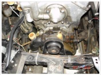
Seems that a previous mechanic had snapped off a bolt in the front engine cover that was used to fasten the water pump and hold an alternator mount. Rather than fixing it properly they just stuck the bolt back in with silicon!! Unbelievable. It must have been leaking for a while based on the what I found upon inspection.
